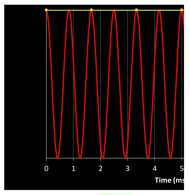
signal frequency = 1200 Hz sample rate = 600 samples per s
